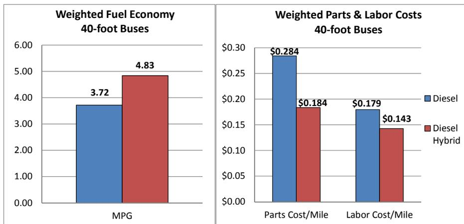
Figure 3-12. Weighted cost and performance comparison for 40-foot buses.
