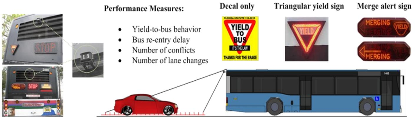
This study focuses on the assessment of the safety and operational benefits of the use of YTB-LED signs on the back of buses. The main objectives of this study are as follows:
