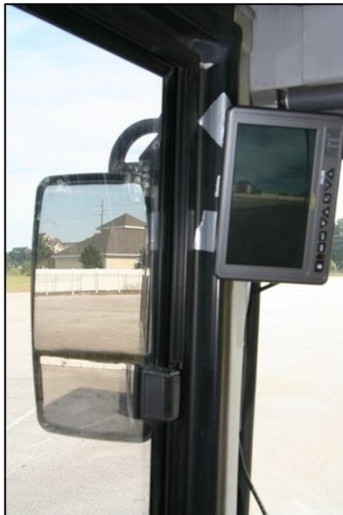
A potential countermeasure to this problem is the use of camera-based systems. The camera-based system for transit buses under evaluation in this study is a system that incorporates video cameras installed on the outside walls of the bus, aimed at the left and right rear sides of the bus, and two monitors connected
