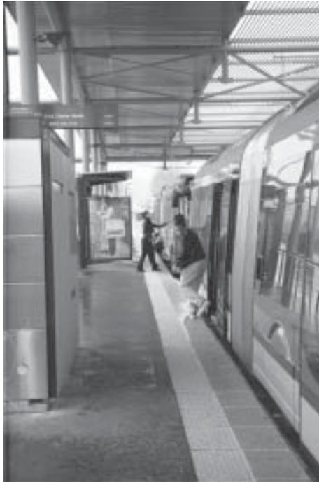
Figure 3 illustrates the docking accuracy possible with electronic guidance systems. Customers easily board and alight from electronically-guided Iris bus Agora and Civis vehicles used on the TEOR System in Rouen, France.
