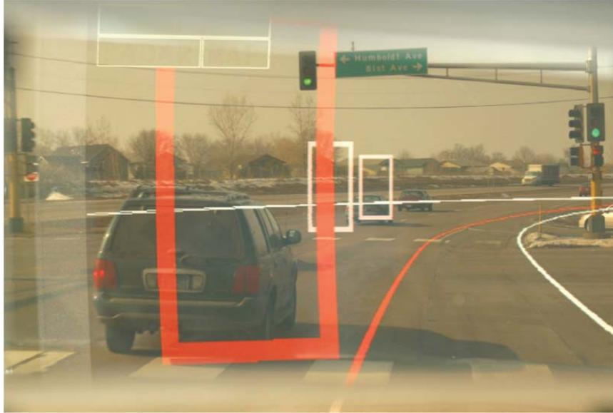
Figure 1 View through MVTA Head-Up Display
